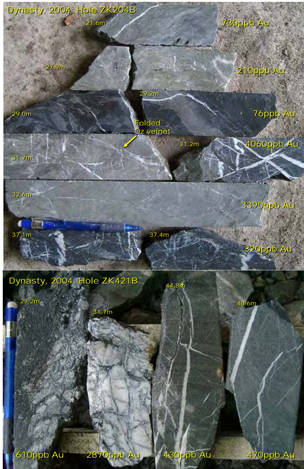
Figure 8. Gold Mineralization Styles at Qi-2. Average Gold Grade as Indicated. Top. Borehole ZK204B. Variably Altered Fine-Grained Sedimentary Rock with Quartz Veining. Bottom. Borehole ZK421B. Quartz Veining Style Hosted in Altered Fine-Grained Sedimentary Rock.
