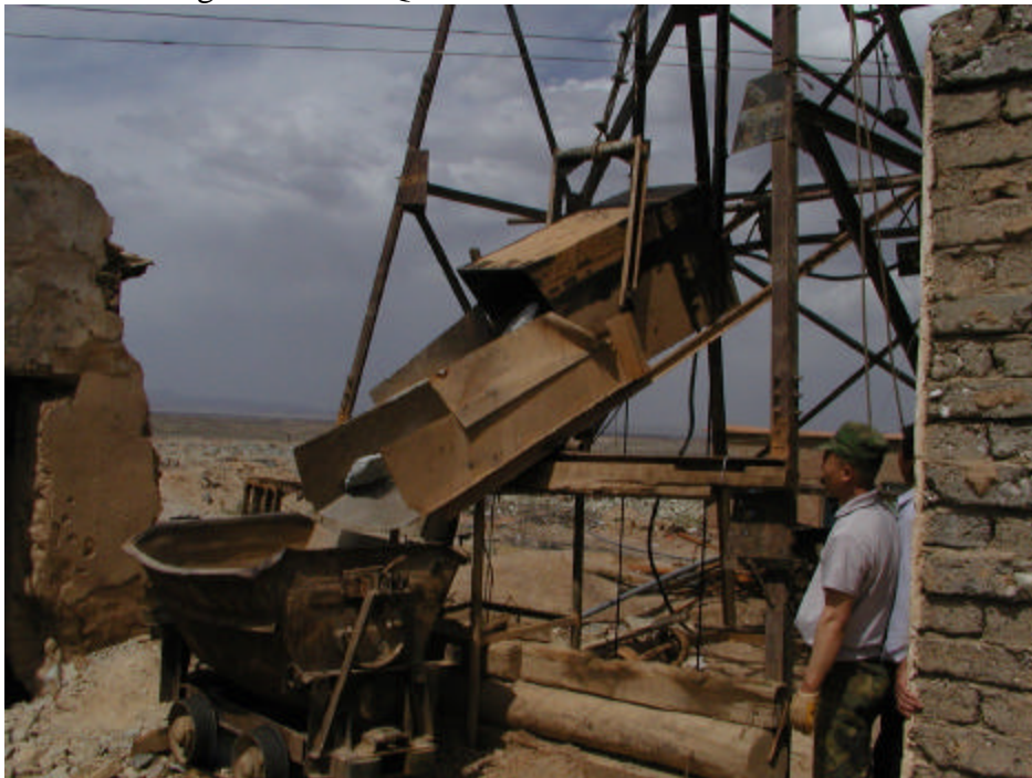
Photo HM-10: Loading ore car at Quartz Vein #49 shaft.
