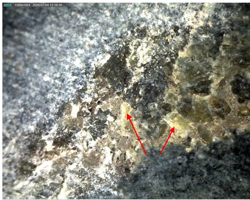
Figure 1: Photo micrograph of drill core from DP26-01 at approximately 100m showing two bright spots (indicated by red arrows) thought to be gold, within a band of pyrite, pyrrhotite, and chalcopyrite. The field of view is 7mm.
